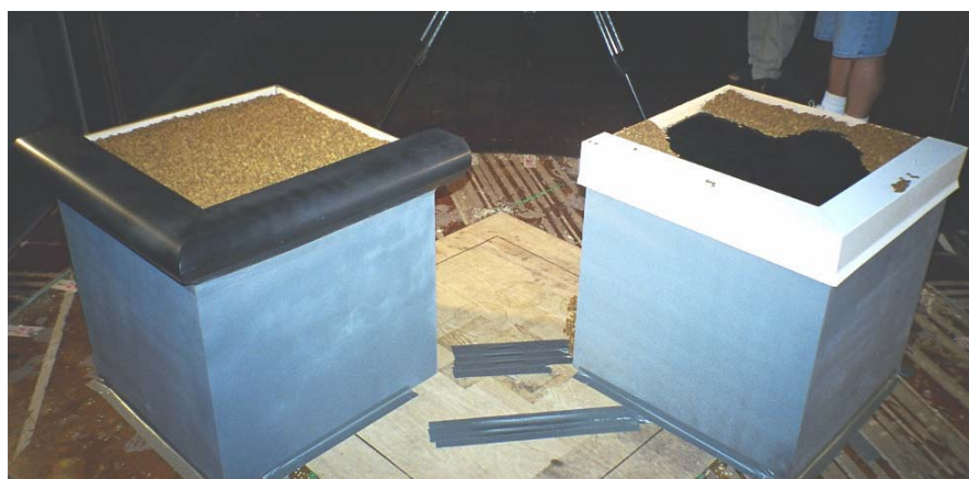
Fig. 5. Wind tunnel test of gravel scour on Aerodynamic edge (left) and Conventional edge
